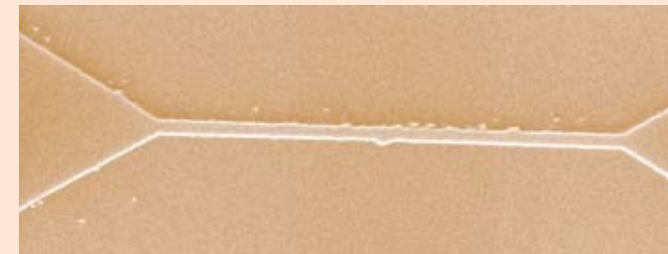
Nano-wire for use in future high density, low power nano-transistors. It could also act as a detector for large molecules in, e.g. biomedical samples. (KTH)
