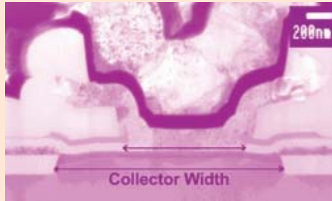
Cross section of a transistor for wireless communication applications in silicon-germanium technology, operating at extremely high frequencies of above 80 GHz. (KTH)
